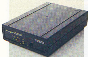
Prism 1000 Type: Hard-wired Viewdata modem Baud Rate: 1200/75 Price: Modem only: £69.95; Full machine-specific package: £129.95
